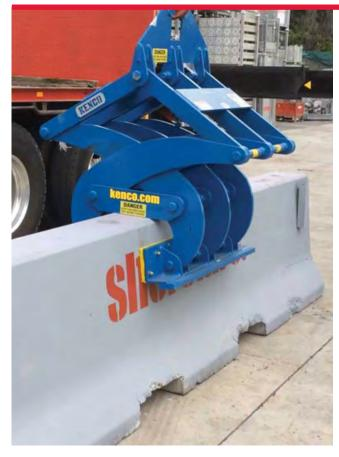
The Kenco Barrier Lifter is a lifting attachment designed to be used in conjunction with our Concrete T-lok Barriers.
