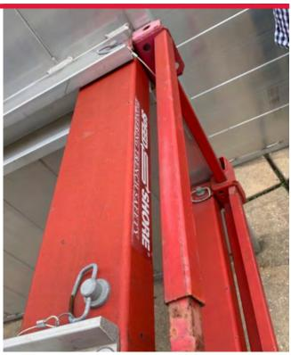
We also offer Trench Sheet Brackets to connect to the end of smoothwall shoring boxes, these brackets allow for easy installation of sheets as end shoring to create a fully enclosed system.
