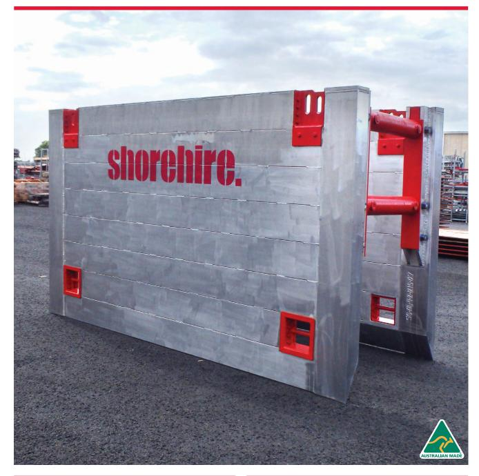
THE 4.2m-60 ALUMINIUM TRENCH BOX IS FOR HEAVY-DUTY, GENERAL PURPOSE SHORING, AND IS SUITABLE FOR MOST EXCAVATIONS AND MACHINES. The 150mm thick panel has been designed to withstand the higher ground pressure needed for large pipe installation, boring pits, pump stations, or projects where long pipe runs are being laid.
