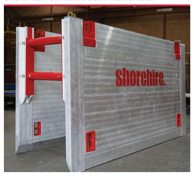
THE SHORE 4.2m-35 ALUMINIUM TRENCH BOX PROVIDES THE PERFECT BALANCE OF STRENGTH, TOUGHNESS AND LIGHT WEIGHT TO ALLOW SMALLER EXCAVATORS TO HANDLE THE REALLY DIFFICULT PIPELINE PROJECTS. With a 100mm wall thickness, the 4.2m-35 Aluminium Trench Box allows for narrower trenches in tight projects and means less bedding material is required which converts to real savings on most pipeline projects.
